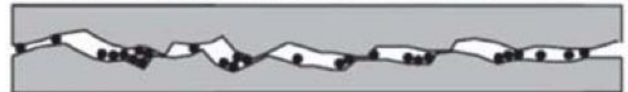
Case 4: Displaced fracture faces, 0.1 lbm/ft 2 proppant
