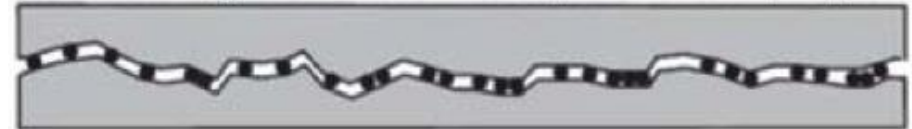
Case 3: Aligned fracture faces, 0.1 lbm/ft 2 proppant
