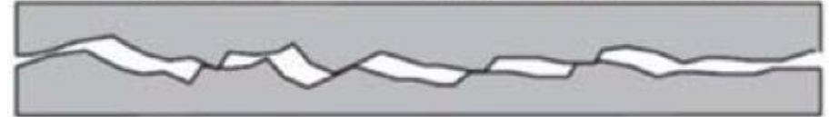
Case 2: Displaced fracture faces, no proppant
